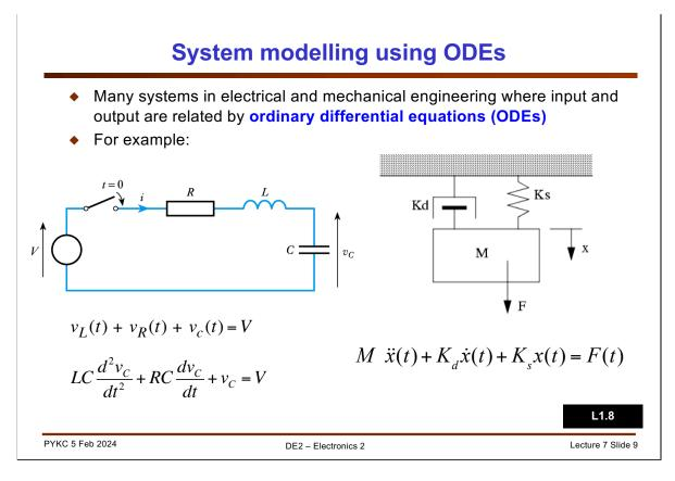
You are familiar with modeling systems with differential equations. Assuming that all voltages and currents were 0 for t < 0. At t = 0, the switch closes. We are interested in find out  $v_c(t)$  as a function of time.
